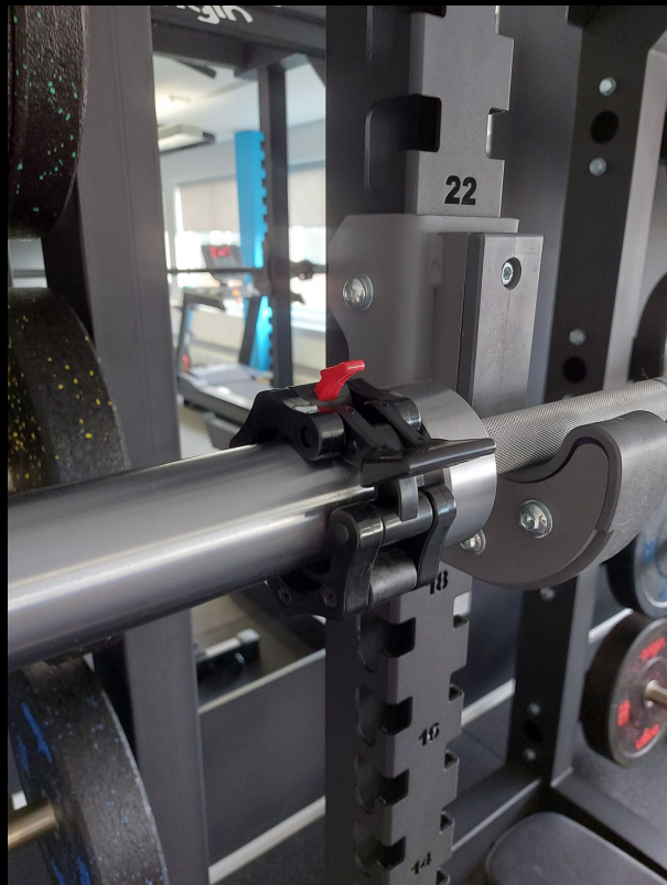
Open (unsafe when loaded)
